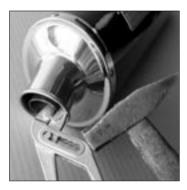
Put a set of adjustable-joint pliers on the Db eater. Tap with a hammer on the pliers and the dB eater will come out.
