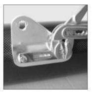
On some models we supply a locking tab to prevent the bolts from coming loose. You have to secure the bolts by folding the tab towards the heads of bolts with pliers.
