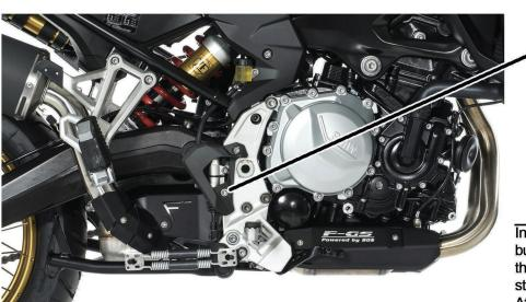
Replace original bolt by Pos.5 Bolt M6x50
